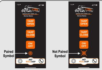
Note: Your Control Box needs to be Powered On for your App to be paired. BlueTooth range is approximately 50-100ft. Large buildings / structures between will interfere with the signal.
